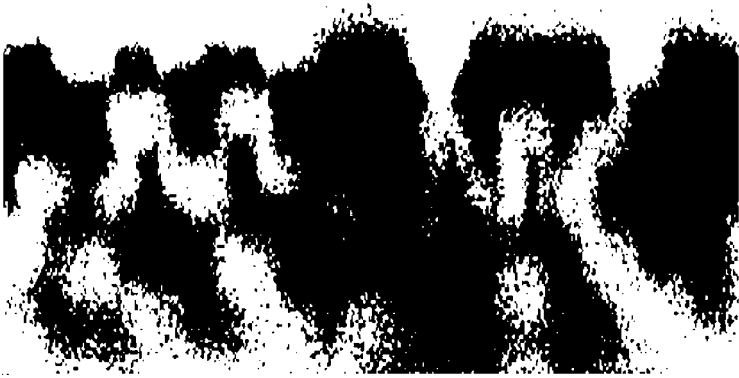
Figure 4.54 A noisy XZ image which has been thresholded and segmented. The surface is at the top of the image and, due to shadowing, fibre images seem to blend into the image of a near neighbour. The scale is 100\ \mu\text{m} \times 50\ \mu\text{m} in XZ.
