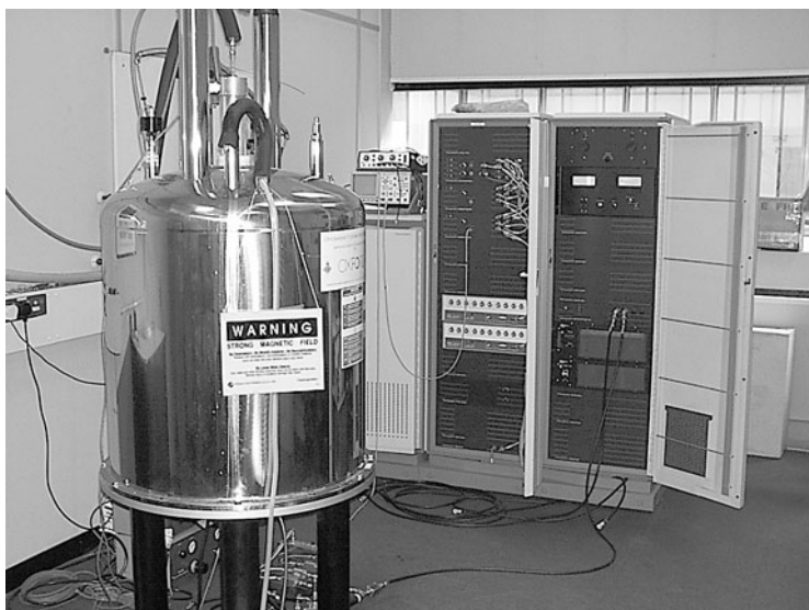
Figure 6.11 A typical nuclear magnetic resonance research system used in the Department of Physics and Astronomy at the University of Leeds. The cryostat ensures that the sample for analysis is kept at sub-zero temperatures.
