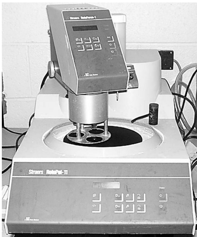
Figure 3.4 One of the polishing machines used in Leeds for sample preparation is the Struers Rotopol-11. Three samples, each potted in epoxy resin, may be polished at the same time.
